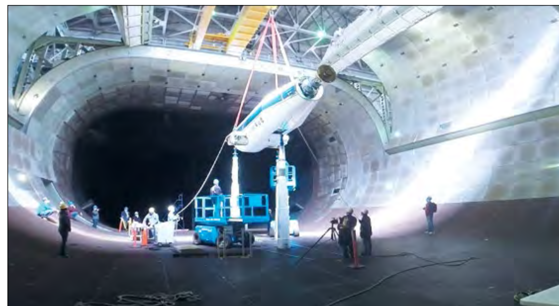
Arnold Engineering Development Complex crew members lower the NASA/Army Tiltrotor Test Rig into the 40-by-80-foot wind tunnel in the AEDC National Full-Scale Aerodynamics Complex at Moffett Field in Mountain View, California. The rig was developed to study advanced tiltrotors and develop databases for design-code validation.
